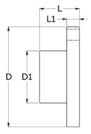
$\begin{array}{lll} D & = 285 \\ D1 & = 164 \\ L & = 110 \\ L1 & = 32 \\ Max bore & = 100 \\ Torque (N m) = 4300 \end{array}$
